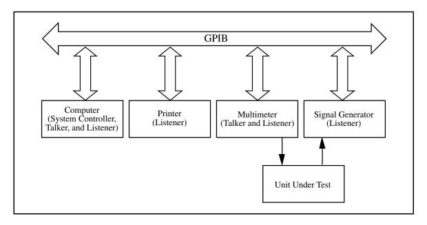
Figure 1-3. Typical GPIB-130 Extension System (Logical Configuration)
