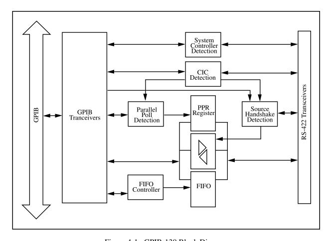
Figure 4-1. GPIB-130 Block Diagram
