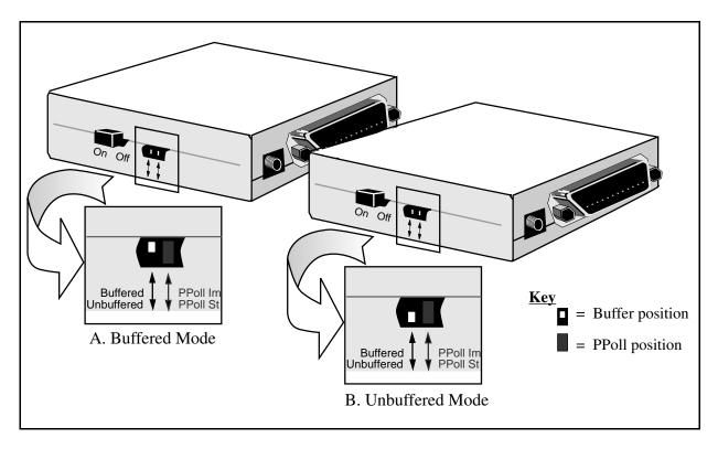
Figure 3-1. Switch Setting for Operating Mode
