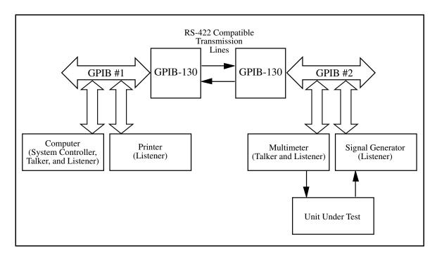
Figure 1-2. Typical GPIB-130 Extension System (Physical Configuration)
