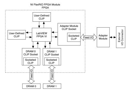
The NI 6587 ships with socketed CLIP items that add module I/O to the LabVIEW project.
