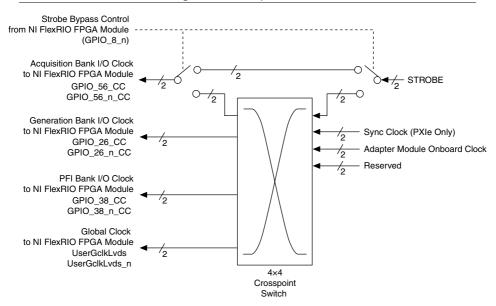
In software, each clock output terminal is accessed with a U8 data type. The following table shows the values of the crosspoint switch clock options.
