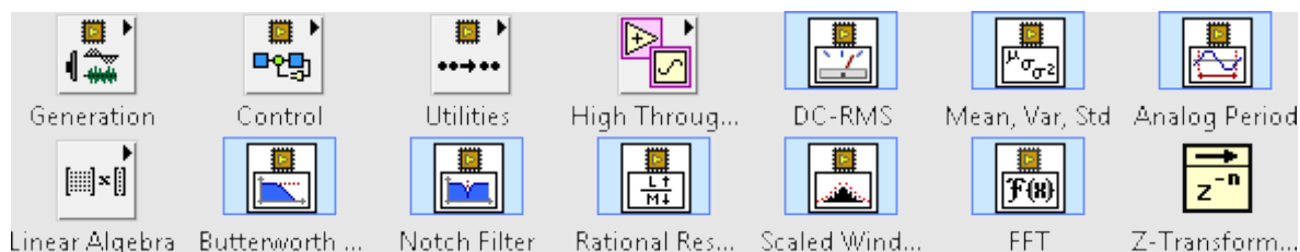
Figure 8. Just one of the palettes of FPGA IP included with LabVIEW FPGA.
