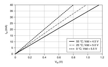
Figure 7. PFI <0..15>/P1/P2: I<sub>ol</sub> versus V<sub>ol</sub>
