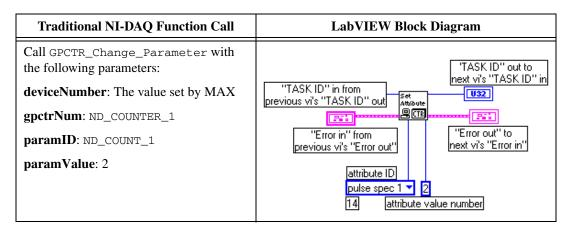
8. Set the pulse width for the single-pulse generation. The following example assumes a 10 MHz source (period = 100 ns) for counter 1. Therefore, the pulse width is 100 ns × 500000 = 50 ms. If you use a frequency other than 10 MHz, adjust the number accordingly. For a frequency F, 1/F × ND\_COUNT\_2 should equal 50 ms.
