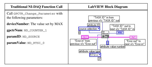
c. Route the stable 10 MHz clock on the PXI-6608 onto RTSI line 0.
