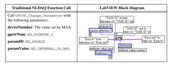
3. Configure the **gate** of counter 0 to be the **output** of counter 1.
