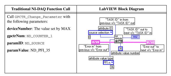
7. Set the pulse delay for the single-pulse generation.
