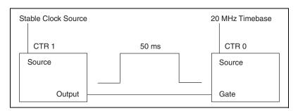
Figure 1. NI 6601/6602 Verification Process
