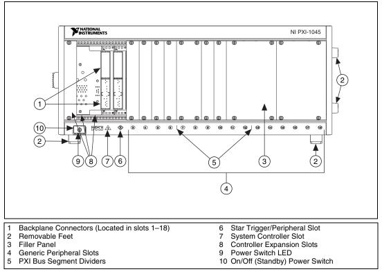
Figure 1-1. Front View of the PXI-1045 Chassis
