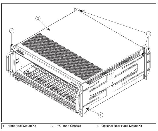
Figure A-3 shows the PXI-1045 rack-mount kit components.
