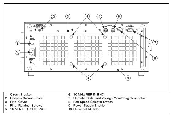
Figure 1-2. Rear View of the PXI-1045 Chassis
