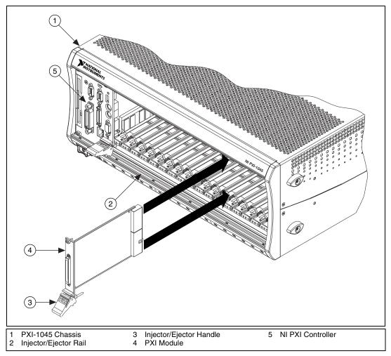
Figure 2-4. Installing PXI or CompactPCI Modules
