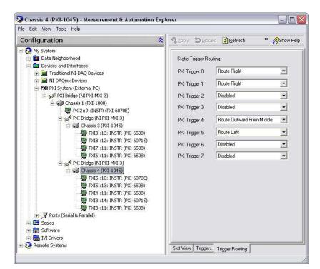
Figure 2-5. Multichassis Configuration in MAX
