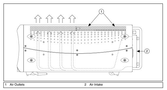
Figure 2-1. PXI-1045 Chassis Airflow Side View
