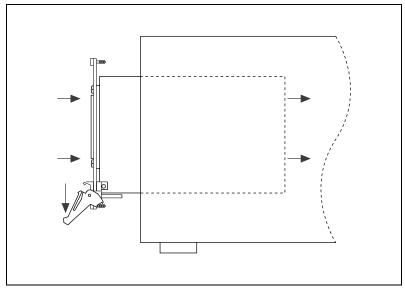
Figure 2-2. Injector/Ejector Handle Position during Controller or Peripheral Module Insertion
