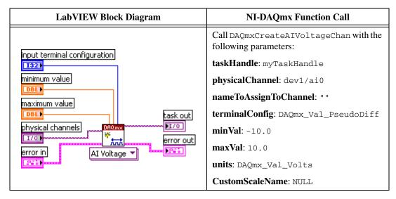
5. Modify the AI voltage channel properties using the following functions.
