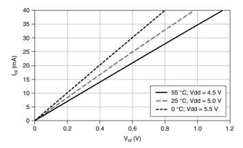
Figure 8. PFI <0..15>/P1/P2:  $I_{ol}$  versus  $V_{ol}$
