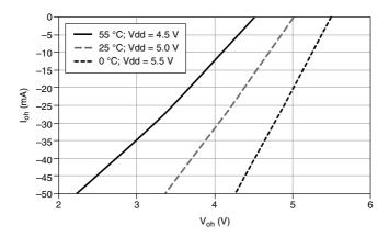
Figure 6. PFI <0..15>/P1/P2:  $I_{oh}$  versus  $V_{oh}$
