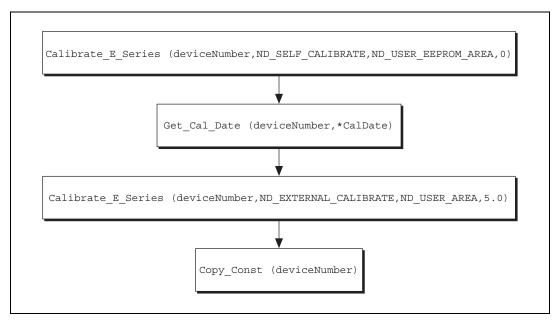
**Figure 3.** Adjusting the NI 6711/6713/6731/6733
