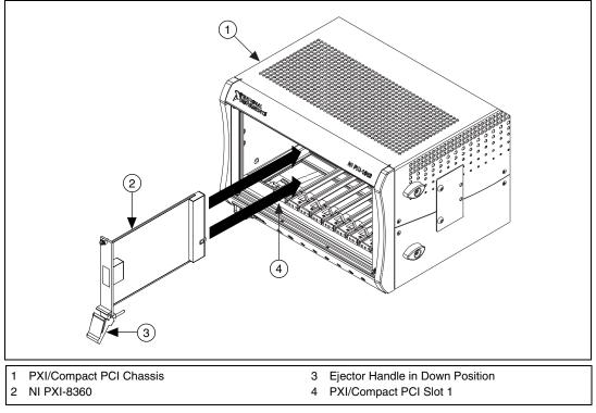
Figure 2. NI PXI-8360 Card Before Installation
