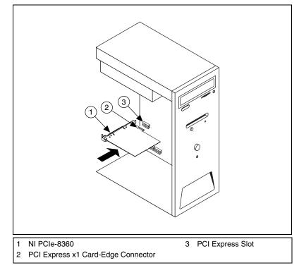
Figure 1. Installing the NI PCIe-8360
