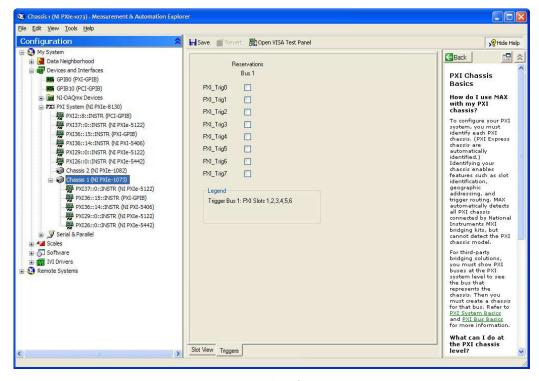
Figure 2-8. Configuring Triggers in MAX
