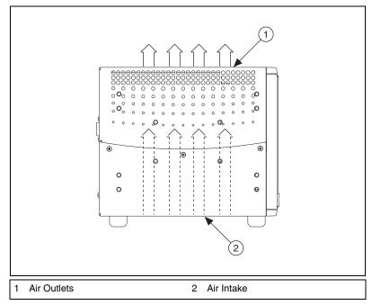
Figure 2-1. NI PXIe-1073 Module Cooling Airflow Side View
