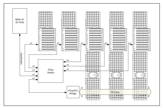
Refer to Figure 1-4 for an overview of the NI PXIe-1073 architecture.
