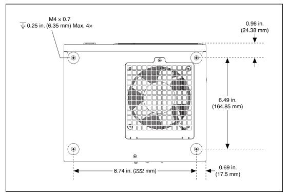
Figure A-2. NI PXIe-1073 Chassis Dimensions (Bottom)
