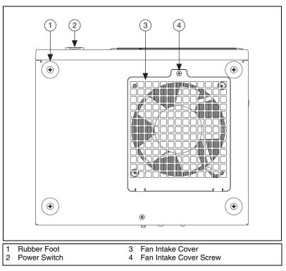
Figure 1-3. Bottom View of the NI PXIe-1073 Chassis
