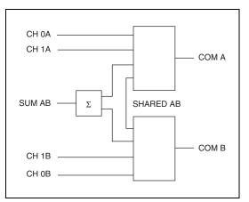
Figure 5. NI PXIe-2790 Hardware Diagram
