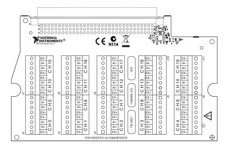
6. Tighten the terminal screws to a torque of  $0.3 \text{ N} \cdot \text{m} (2.7 \text{ lb} \cdot \text{in.})$ .
