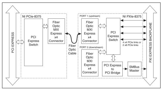
Figure 3-1. Fiber-Optic MXI-Express x4 Block Diagram
