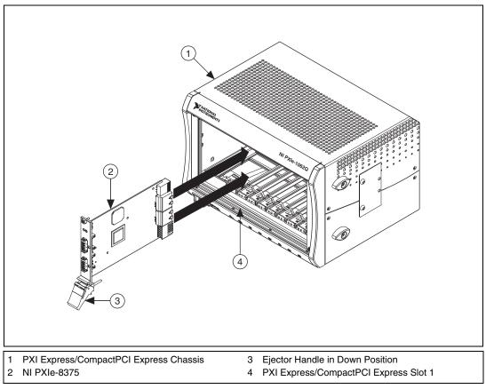
Figure 2-2 shows an NI PXIe-8375 just before installation in the system controller slot of a National Instruments PXI Express chassis.
