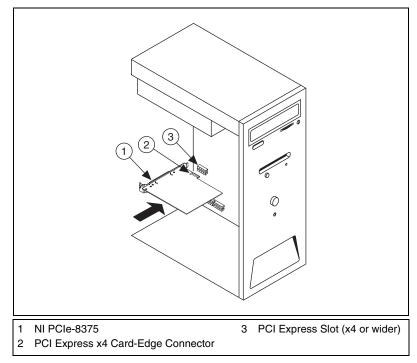
Figure 2-1. Installing the NI PCIe-8375
