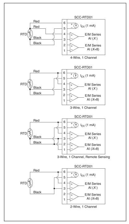
Figure 1. SCC-RTD01 Single-Channel Wiring Diagrams
