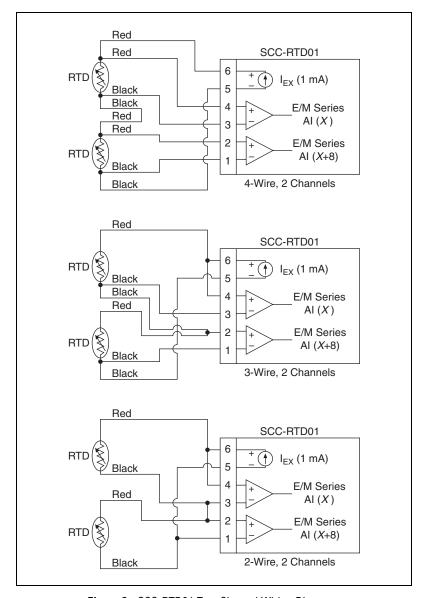
Figure 2. SCC-RTD01 Two-Channel Wiring Diagrams
