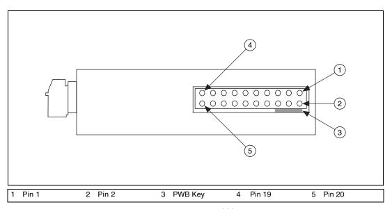
Figure 4. SCC Module Bottom View
