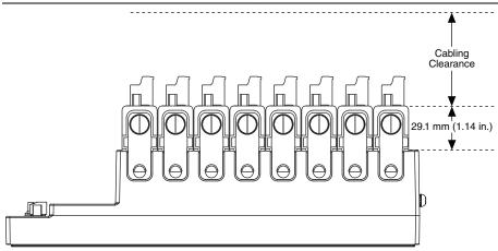
Measure the ambient temperature at each side of the cDAQ chassis, 63.5 mm (2.50 in.) from the side and 38.1 mm (1.50 in.) forward from the rear of the cDAQ chassis, as shown in the following figure.
