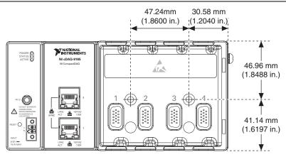
Figure 1-21. cDAQ-9189 Surface Mounting Dimensions
