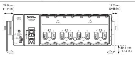
Figure 1-30. Desktop Mounting Side Dimensions
