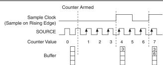
Figure 6-4. Buffered (Sample Clock) Edge Counting
