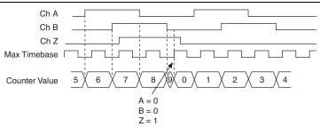
Figure 6-20. Channel Z Reload with X4 Decoding
