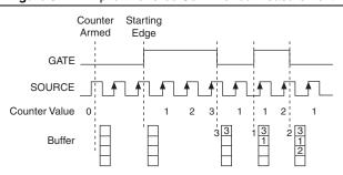
Figure 6-11. Implicit Buffered Semi-Period Measurement
