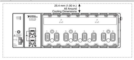
Allow the appropriate space in front of C Series modules for cabling clearance, as shown in the following figure. The different connector types on C Series modules require different cabling clearances. For a complete list of cabling clearances for C Series modules, visit ni.com/info and enter the Info Code crioconn.
