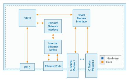
Figure 1-33. cDAQ-9185/9189 Chassis Block Diagram
