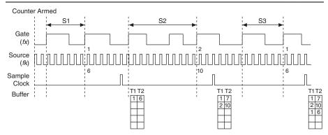
Figure 6-15. Sample Clocked Buffered Frequency Measurement (Averaging)
