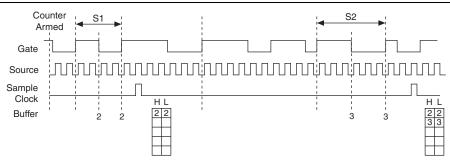
Figure 6-10. Sample Clocked Buffered Pulse Measurement
