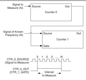
Next, route the Counter 0 Internal Output signal to the Gate input of Counter 1. You can route a signal of known frequency (*fk*) to the Counter 1 Source input. Configure Counter 1 to perform a single pulse-width measurement. Suppose the result is that the pulse width is *J* periods of the *fk* clock.
