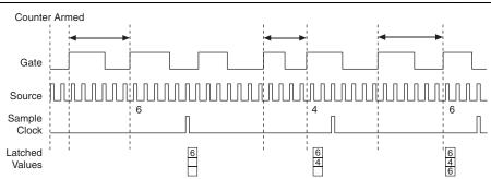
Figure 6-16. Sample Clocked Buffered Frequency Measurement (Non-Averaging)
