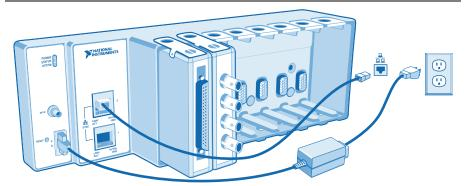
The POWER and STATUS LEDs light. The POWER LED lights as long as power is being supplied to the cDAQ chassis. The STATUS LED turns off after firmware boots. Refer to the *LEDs* section for information about the LEDs on the cDAQ chassis.
