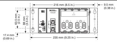
Figure 1-25. cDAQ-9189 Panel Mounting Dimensions
