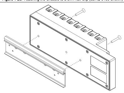
You must use the screws provided with the NI DIN rail kit because they are the correct depth and thread for the DIN rail clip.
