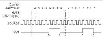
Figure 6-30 shows the same pulse train with CO.EnableInitalDelayOnRetrigger set to the default False.
