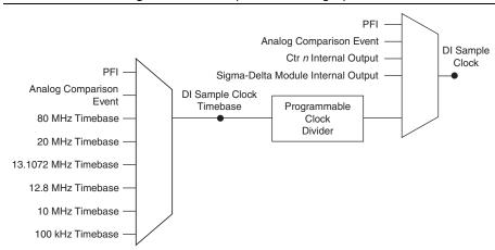
Figure 5-1. DI Sample Clock Timing Options
