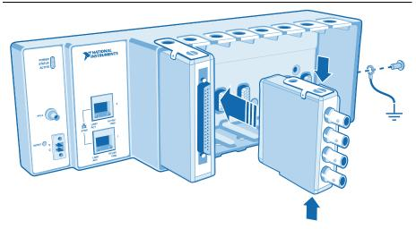
11. Wire the C Series module as indicated in the C Series module documentation.
