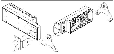
Repeat steps 2 and 3 to attach the other end bracket to the other end of the chassis. 5.
