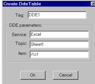
Figure 18-29. DdeTable Definition Parameters Dialog Box (Same Computer)
