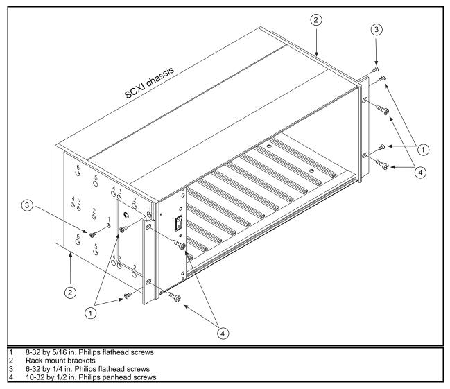
Figure 1. SCXI-1370 Rack-Mount Bracket Installation
