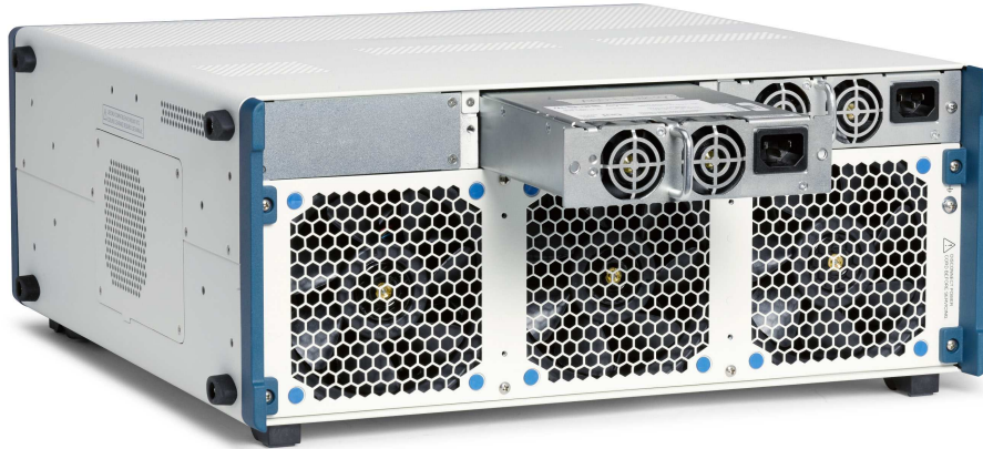
Figure 4: PXIe-1095 power supplies are easily replaceable from the rear of the chassis.
