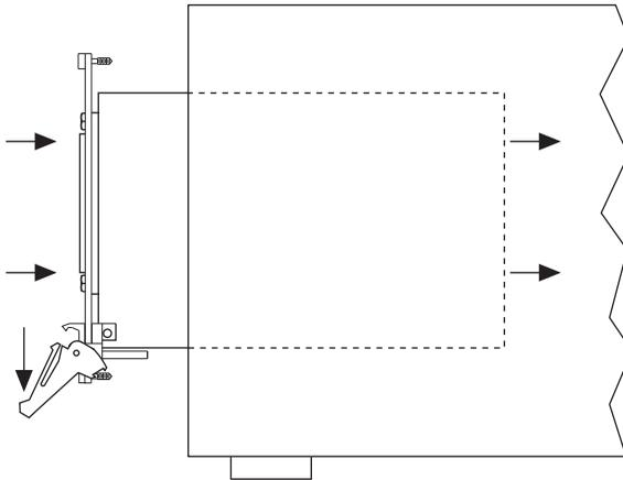
3. When you begin to feel resistance, push up on the injector/ejector handle to inject the controller fully into the chassis frame. Secure the controller front panel to the chassis using the controller front-panel mounting screws.
