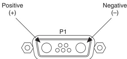
To build a custom DC cable, be sure to note the positive (+) and negative (–) terminals shown in Figure 2-2. Use the following components or their equivalents to mate to the P1 port:
