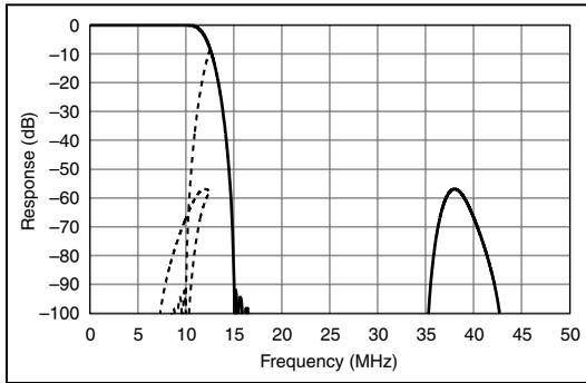
**Figure 6.** DDC Filter Performance, 20 MHz Span
