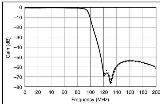
Figure 2. Input Frequency Response for Both Channels (Broadband)
