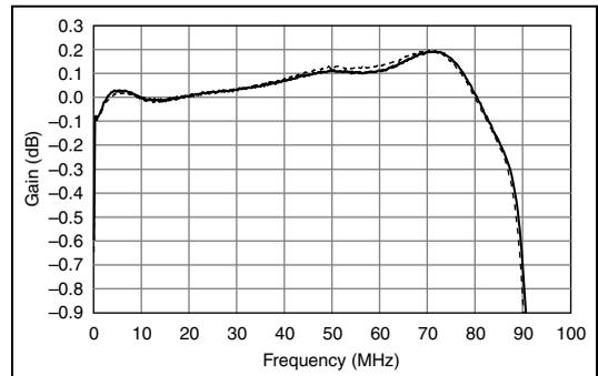
**Figure 8.** Analog Output Passband Flatness
