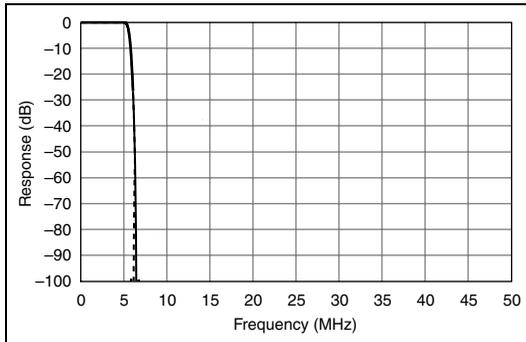
**Figure 7.** DDC Filter Performance, 10 MHz Span
