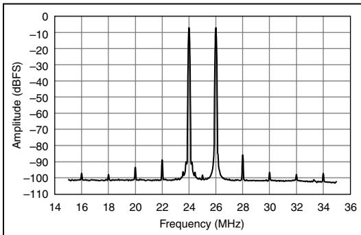
**Figure 4.** Analog Input Two-Tone Intermodulation Distortion (IMD)
