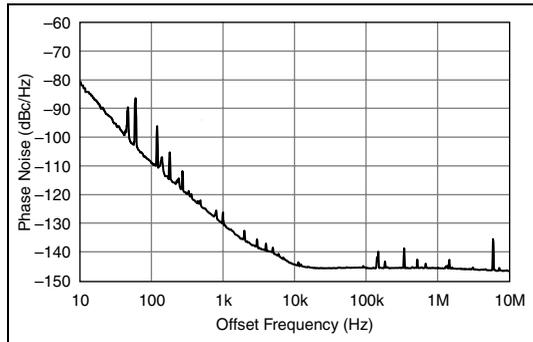
**Figure 5.** Phase Noise at Carrier Frequency = 68.659 MHz
