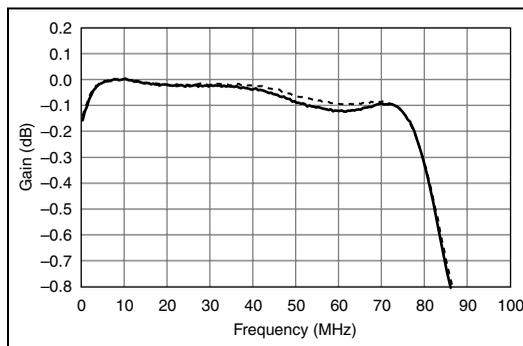
Figure 1. Input Frequency Response for Both Channels (Passband)
