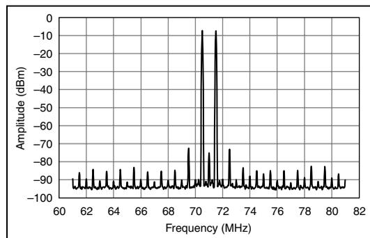
**Figure 12.** System-Level Two-Tone IMD,
