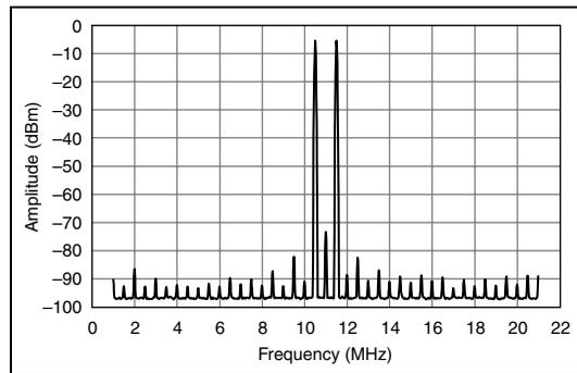
**Figure 11.** System-level Two-Tone IMD,
