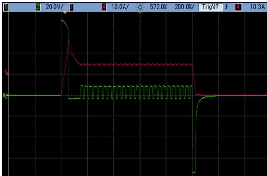
Figure 10. Current and Voltage Traces from Phase1FirstPeakEnable=TRUE Operating Mode
