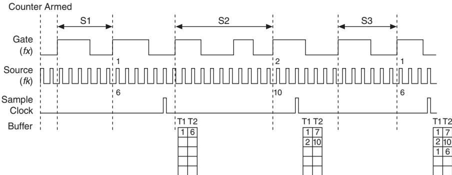
When **CI.Freq.EnableAveraging** is set to false, the frequency measurement returns the frequency of the pulse just before the sample clock. This single measurement is a single frequency measurement and is not an average between clocks as shown in Figure 6-16.
