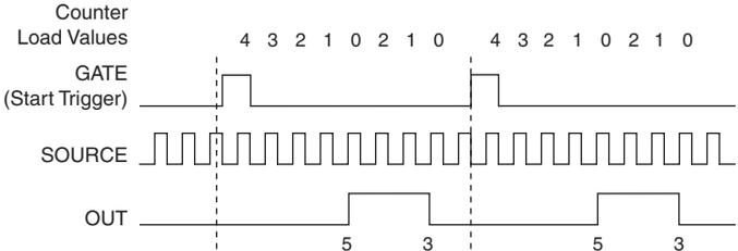
Figure 6-30 shows the same pulse train with **CO.EnableInitialDelayOnRetrigger** set to the default False.
