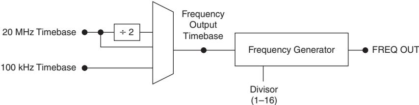
The frequency generator generates the Frequency Output signal. The Frequency Output signal is the Frequency Output Timebase divided by a number you select from 1 to 16. The Frequency Output Timebase can be either the 20 MHz Timebase, the 20 MHz Timebase divided by 2, or the 100 kHz Timebase.
