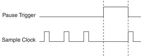
If you are using any signal other than the onboard clock as the source of the sample clock, the generation resumes as soon as the pause trigger is deasserted and another edge of the sample clock is received, as shown in Figure 4-3.
