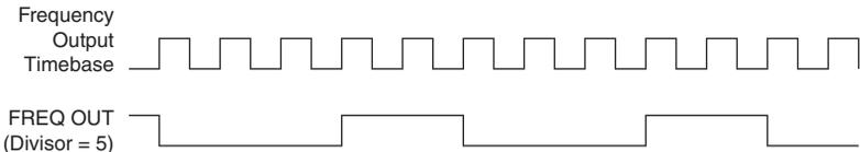
Frequency Output can be routed out to any PFI terminal. All PFI terminals are set to high-impedance at startup. The `FREQ OUT` signal also can be routed to many internal timing signals.
