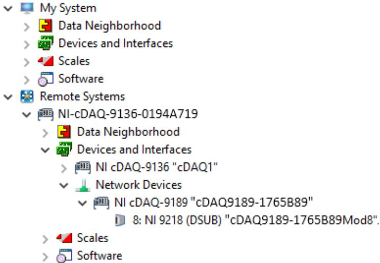
12. Self-test your chassis in MAX by expanding the real-time controller»**Devices and Interfaces**»**Network Devices**, right-clicking **NI cDAQ-<model number>**, and selecting **Self-Test**. Self-test performs a brief test to determine successful chassis installation. When the self-test finishes, a message indicates successful verification or if an error occurred. If an error occurs, refer to [ni.com/support/daqmx](https://ni.com/support/daqmx).
