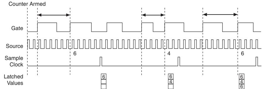
With sample clocked frequency measurements, ensure that the frequency to measure is twice as fast as the sample clock to prevent a measurement overflow.
