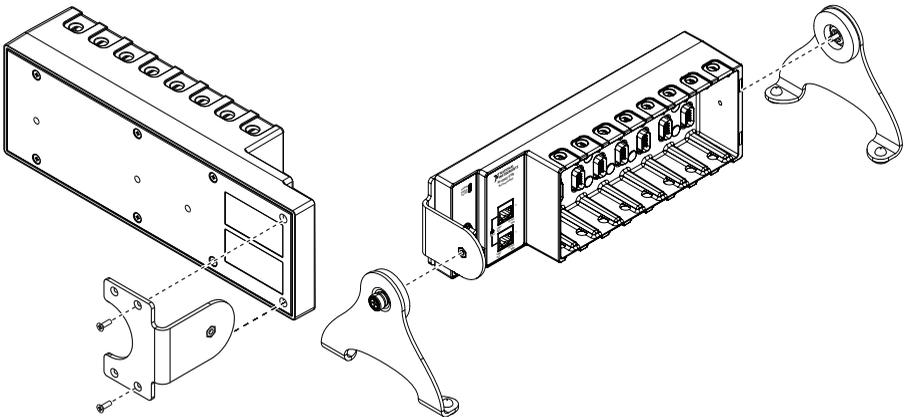
5. Repeat steps 2 and 3 to attach the other end bracket to the other end of the chassis.
