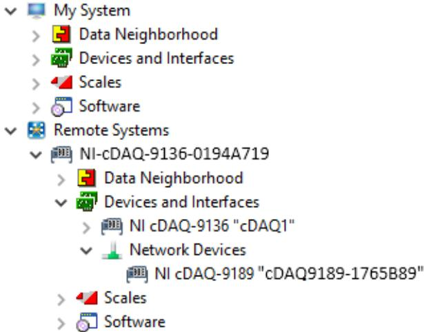
11. If the cDAQ chassis is not reserved automatically, select the chassis and click the **Reserve Chassis** button. Refer to the [Reserving the Chassis in MAX](#) section for more information. After the chassis is reserved by the real-time controller, the modules in the chassis are visible in the MAX configuration tree.
