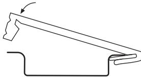
3. Insert one edge of the DIN rail into the deeper opening of the DIN rail clip.
