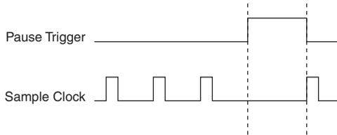
If you are using any signal other than the onboard clock as the source of the sample clock, the generation resumes as soon as the pause trigger is deasserted and another edge of the sample clock is received, as shown in Figure 5-6.
