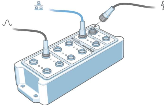
Connect Ethernet Port 0 on the FieldDAQ to a network port or directly to the network card in your computer. Then connect the power supply to the Power IN Port.
