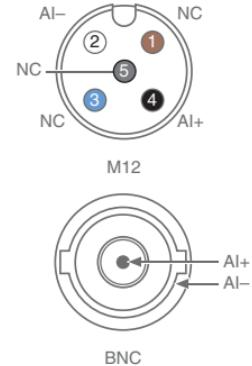
Connect signals to the FieldDAQ. For M12-BNC cables, AI+ routes to the BNC pin and AI- routes to the BNC shield. Refer to the user guide for complete signal connection information.
