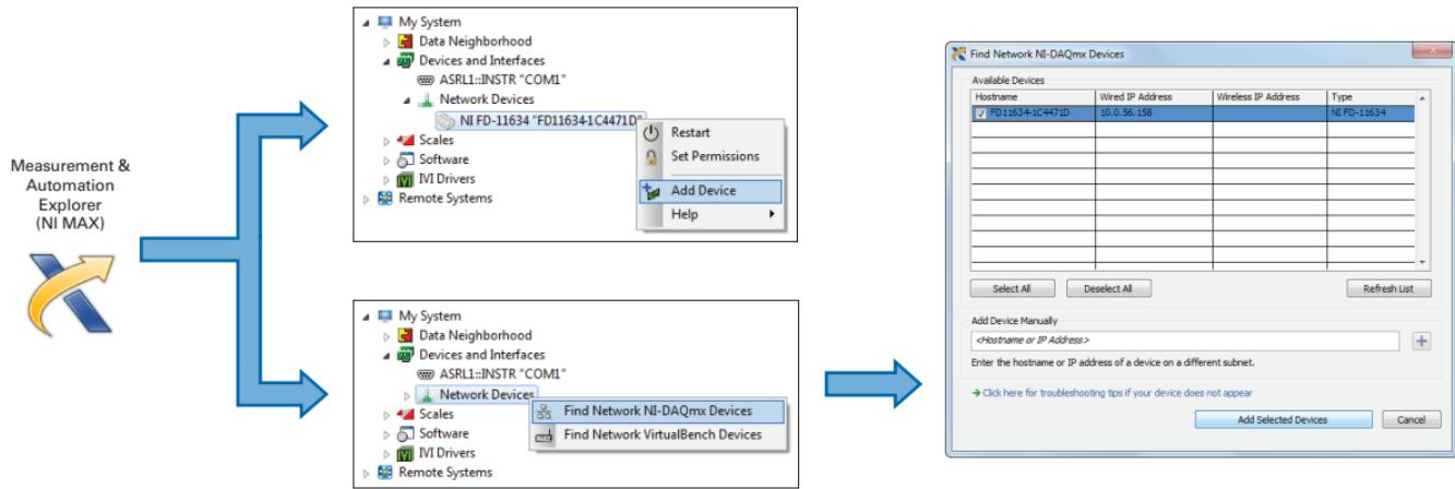
Open MAX. If the device is listed, right-click it and select **Add Device**. If it is not listed, right-click **Network Devices** and select **Find Network NI-DAQmx Devices**. Select a device or manually enter the hostname or IP address. Click the troubleshooting link for help.
