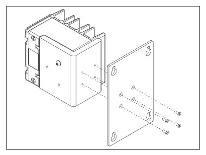
2. Bolt or screw the panel-mount plate to a panel. The following figure shows the dimensions of the controller with the panel-mount plate attached.
